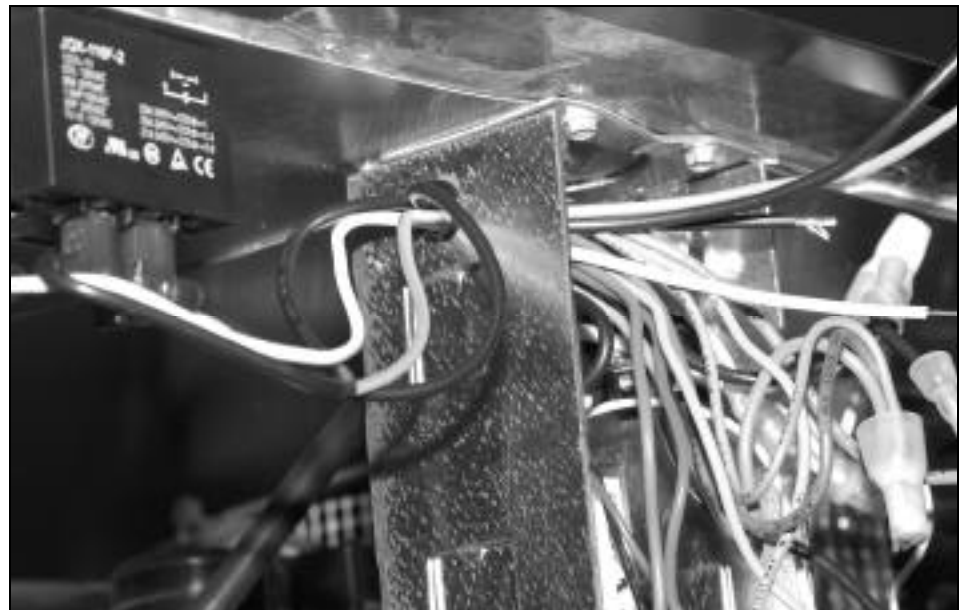
Figure 7. Routing relay wires
